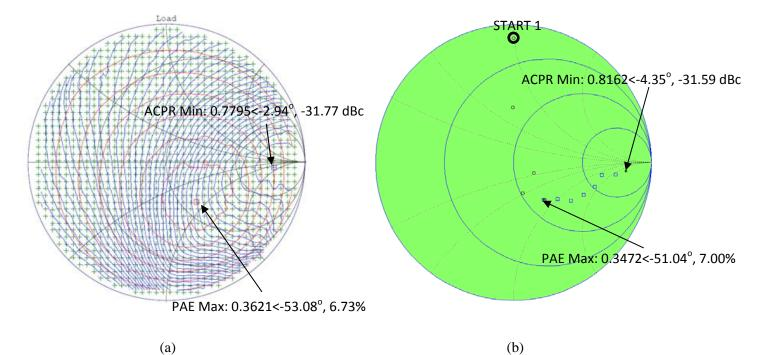
Figure 1: Traditional Load-Pull with 1000 Queries (a) and Sequential Steepest Ascent for PAE (circle) and ACPR (square) with 46 Queries (b)
